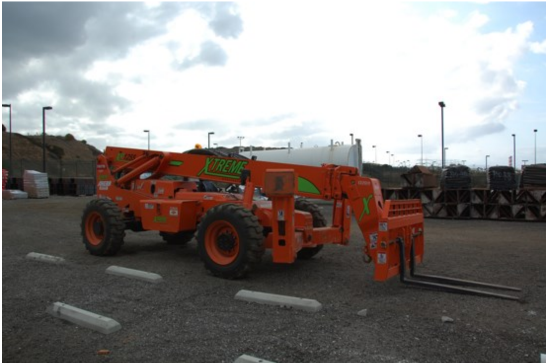
Figure 1.2.2-3: Tier 4i Construction Equipment Utilized on Taxilane T
