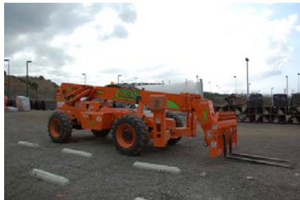
Tier 4i Construction Equipment Utilized on Taxilane T
